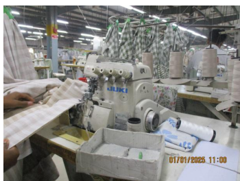
NC photo_Eye guard displaced from actual position.JPG
