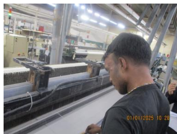
NC photo_Ear plug not used by weaving machine operators.jpg
