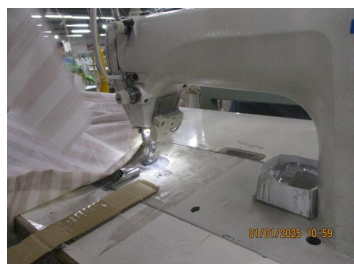
NC photo_Needle guard missing at plain sewing machine.JPG
