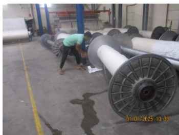
NC photo_No safety shoes used by workers at loading unloading heavy beams.jpg
