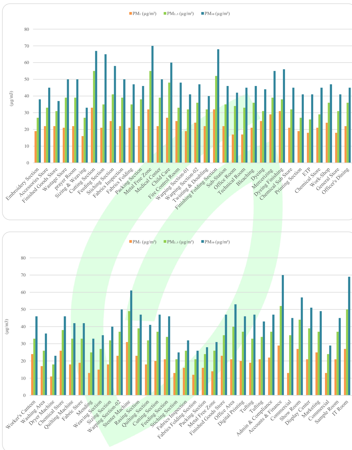
Figure: Indoor Particulate level Monitoring Chart
